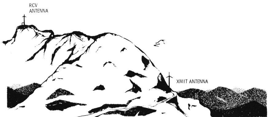
Fig. 4-33. Site layout for on-channel repeater. On-channel capability exists when the transmitting and receiving antennas are poorly situated with respect to each other, though both are adequately positioned for coverage in the general area of use. The Radio Ranch repeater antennas are separated by a mountain of rock rendering the receiver immune to low-power signals from the transmitter.
