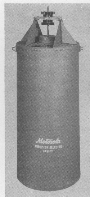
Fig. 4—Quarter-wave cavity selector used for base station control of intermodulation and desensitizing in the 160-Mc band.
