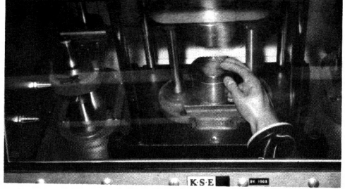
Crystals for special high-precision use get the Coldweld treatment (above) before final inspection (below)
