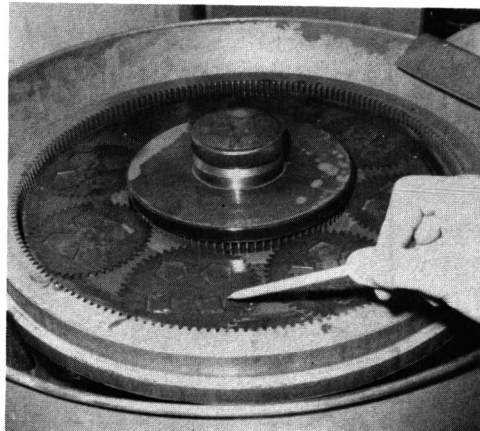
Following the x-ray, each crystal is loafed and rounded (above), then transferred to another department for lapping and calibration (below).
