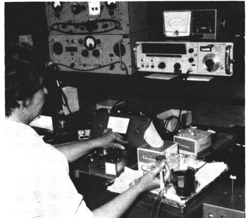
The crystal is mounted and bonded to a base fixture.
