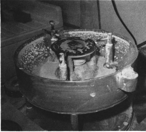
Some high-frequency crystals need a high-speed polish.
